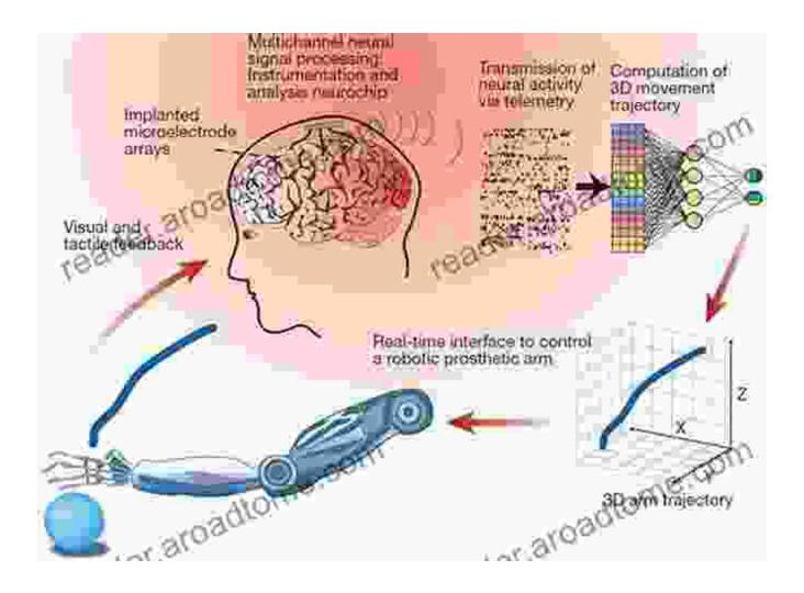
Somatosensory feedback completes the communication loop between the user, neuroprosthesis, and environment.
